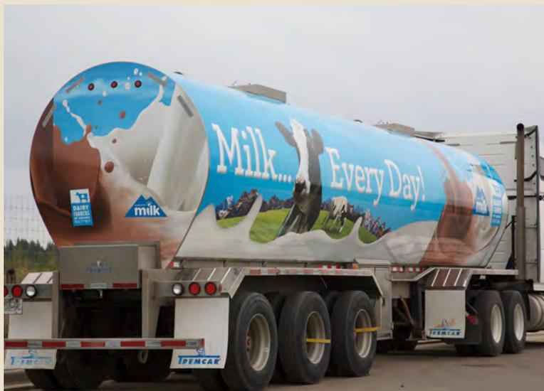
Milk is transported from the farm to the processing plant in special stainless steel insulated tankers (big trucks).
